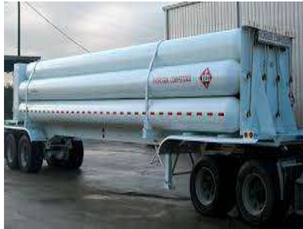
Fig 4: Compressed Hydrogen Gas Tube Trailer – 30 Cylinders and 43,260 SCF (105 kg) capacity.
