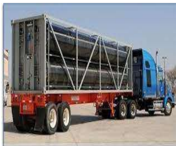
Fig 6: Next Generation Hydrogen Delivery System Undergoing Testing
