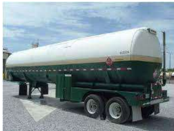
Fig 5: Cryogenic Liquid Hydrogen Trailer – 13,000 gallon (3,500 kg) capacity.
