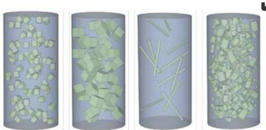
Figure 9. Examples of mechanical recycling infill in concrete samples
