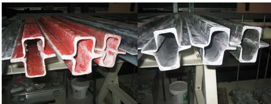
Figure 10. Examples of beam patterns made from virgin and partially recycled GFRP material
