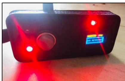
Figure 3 Gas Leakage Detector
