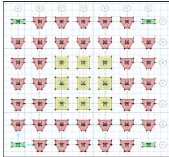
Fig.7. Optimized Pile Foundation
