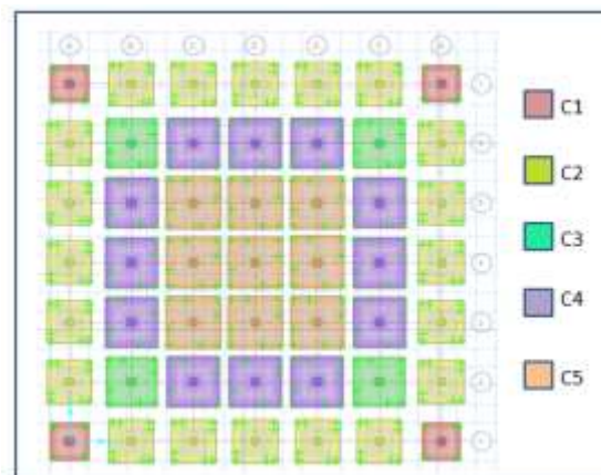
Fig.4. Optimized Isolated Footing
