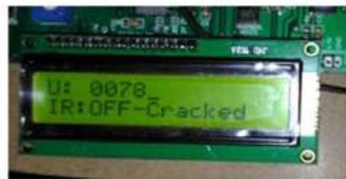
Figure12: Distance from Opposite Vehicle and Crack on Track
