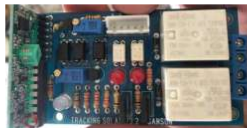
Figure 7. The navigation circuit
