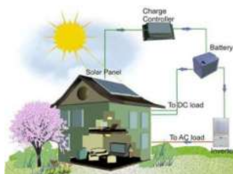
Figure 1. Working principle of solar battery
