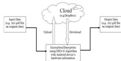
Fig.2 Proposed System Architecture
