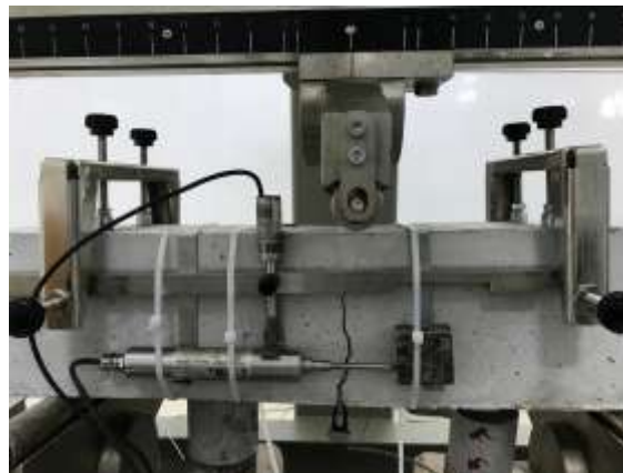
Three-point bending test of high-quality concrete samples using steel fibers
