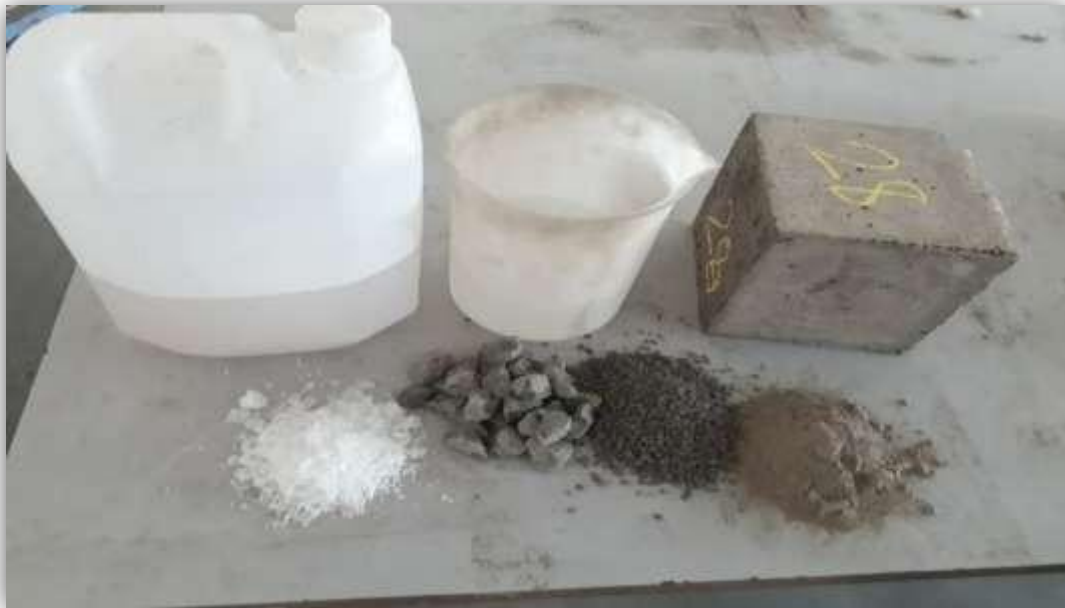
Fig.1. Material used in fly ash Concrete.
