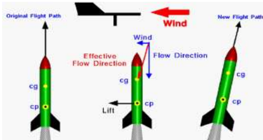
Fig 5: Represents the inclination due to weather cocking [15]
