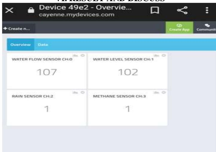
Figure 3. Measurement of Sewer Clogging
