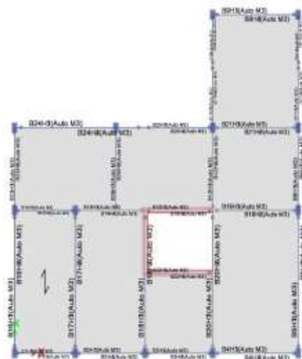
Fig.10.4 Assigned auto hinges in beam
