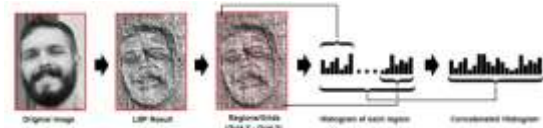
Figure 5: Diagram showing the formation of histogram from the the X and Y grids which is obtained from the LBP result
