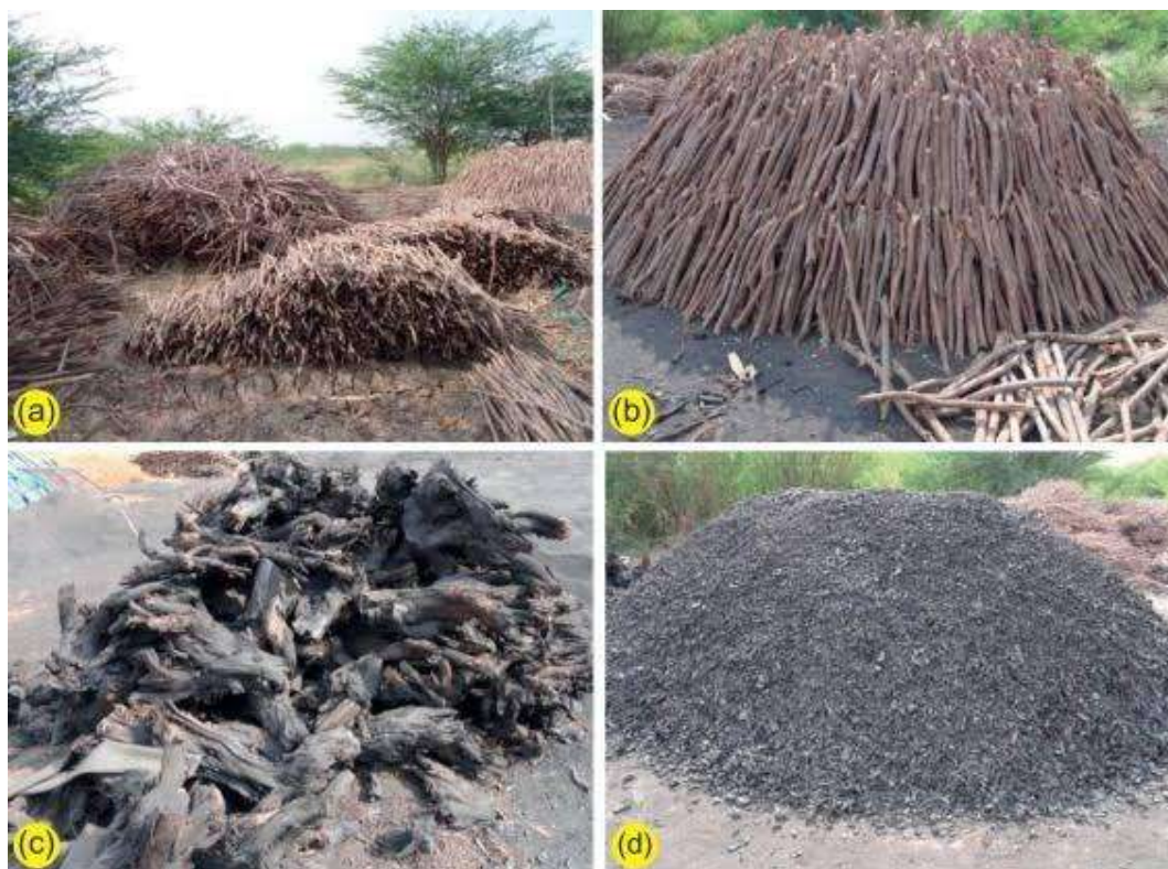
Charcoal production from Prosopis juliflora a) harvested stem wood lots b) harvested wood arranged for controlled burning c) charcoal from root wood and d) charcoal final product ready for domestic and industrial use.
