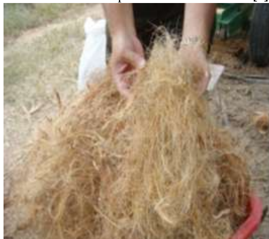
Plate Error! No text of specified style in document.-4: Coir fiber from coconut husks [5]
