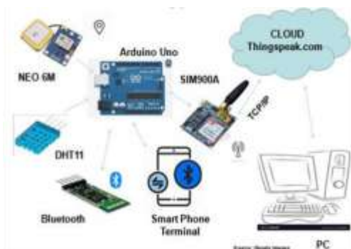
Figure 1. The conceptual block diagram of the IoT Enabled Temperature and Humidity Sensing Device
