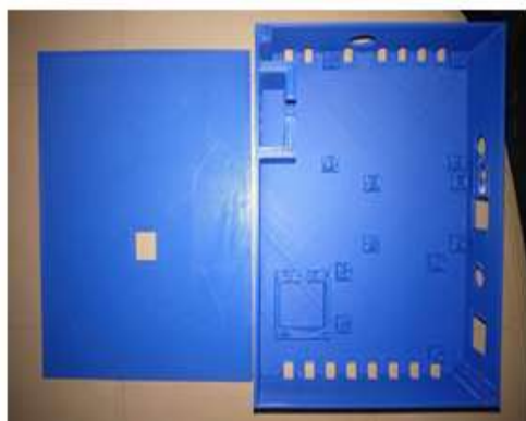
Figure 5. (b) Custom designed and 3D printed enclosure.
