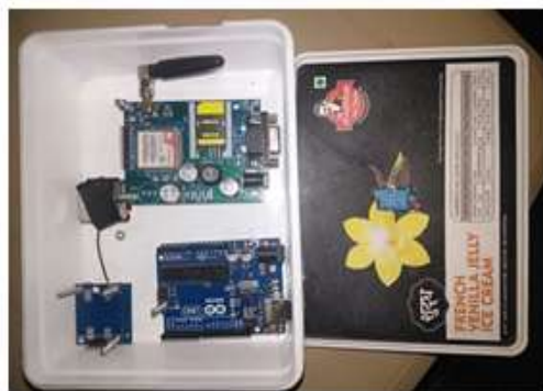
Figure 5. Implementation of the final Prototype Product; (a) ice-cream container used as enclosure.
