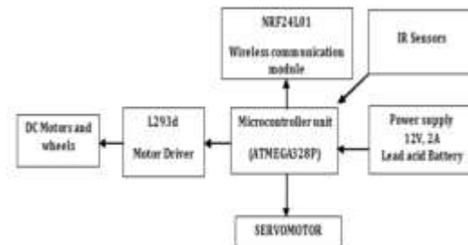
Fig: Block diagram of the swarm robotic system
