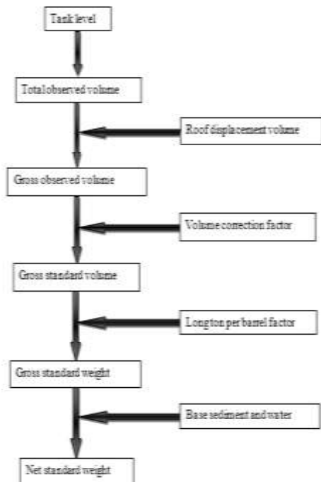
Figure 2: Quantity of mass calculation flow chart
