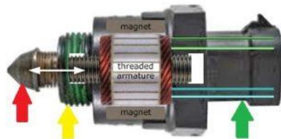
This image shows the inner workings of a typical Idle Air Control valve. In this example, the red arrow indicates the valve pintle, the yellow arrow indicated the threads that mount this particular example on the throttle body, and the green arrow indicates the electrical connector.
