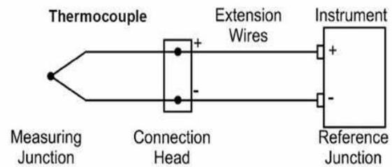
A **thermocouple** is a sensor for measuring temperature. This sensor consists of two dissimilar metal wires, joined at one end, and connected to a thermocouple thermometer or other thermocouple-capable device at the other end. When properly measurements over wide range of temperatures.
