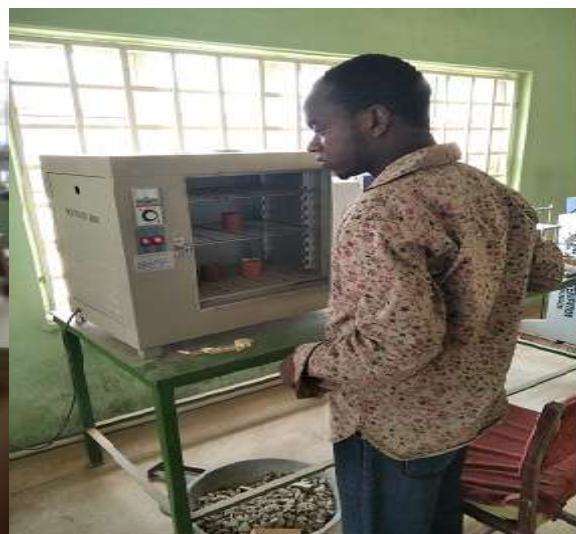
Plate 3: Standard cylindrical Sand samples in a furnace
