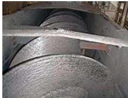
Figure 4.2. Only part of the hard surface of the screw is "polished".
