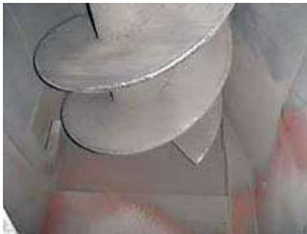
Figure 4.1. The screw conveyor is made with CeraMetal's hard surface material
