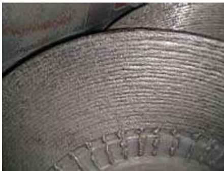
Figure 4.3. The surface of the conveyor screw is "polished"
