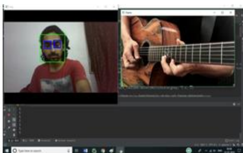
Fig-6 : Face and eyes are detected so media player is playing the video While the face and eyes are detected so the first counter value is 1 so the media player is playing the video
