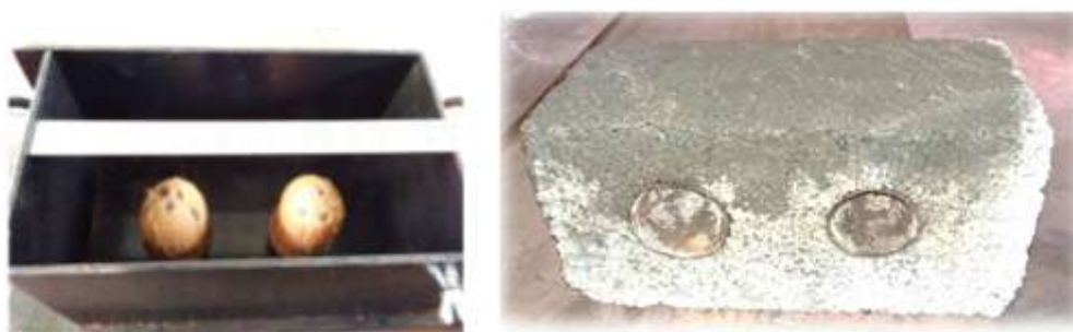
Fig.3.1. (b) Placing the coconut shells in the mould Fig.3.1. (c) The photograph of the bottom portion of the moulded open graded hollow concrete block
