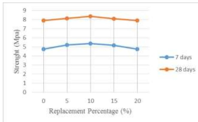
**Fig 5.3: Dolomite powder flexural strength test results**
