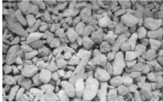
Demolished Coarse Aggregate .
