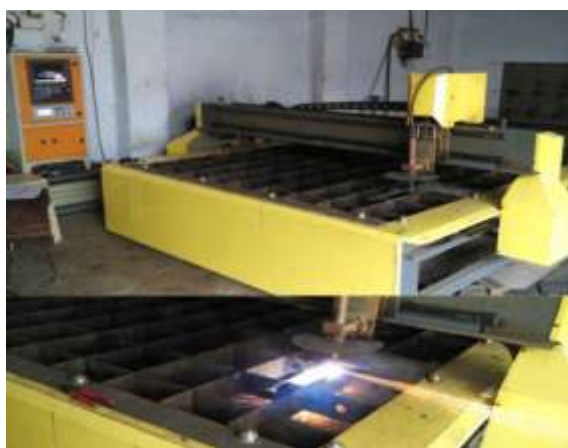
Figure 3.2: Hypertherm powermax 105 CNC machine
