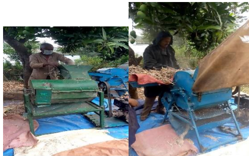
Fig.1. a. Jimma Replaceable Drum Multi Crop Thresher b. Jimma Rice Thresher
