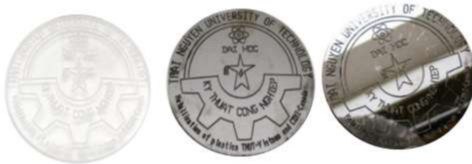
Figure 4: Nickel plating on logo by Plexiglass; (a) before plating; (b, c) after plating
