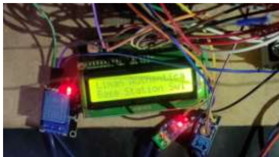
Step 3: Display to show lineman authentication base station switching that is lineman after sensing his finger through fingerprint scanner.
