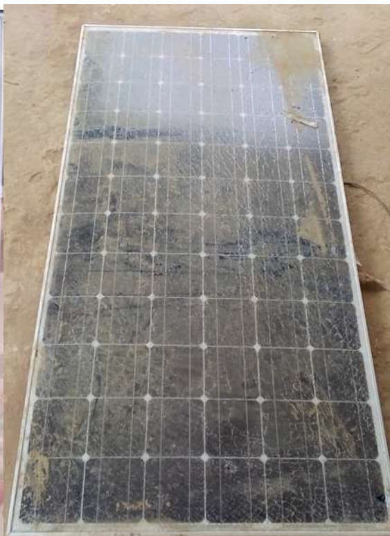
Figure: 3. Dusty Solar module
