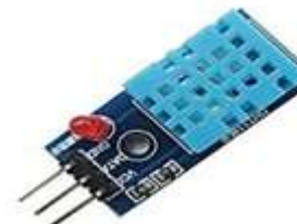
Figure 3.3.2. DHT 11 humidity and temperature sensor
