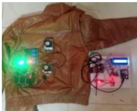
Fig 18: LED indication on hyperthermia condition
