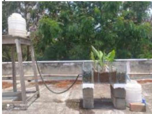
Figure 3. Photographic view of experimental flow Front View of Wetland Pond After plantation
