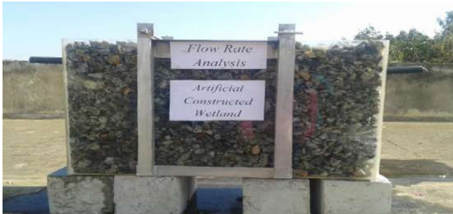
Figure 2. Photographic view of experimental flow Front View of Wetland Pond Before plantation.
