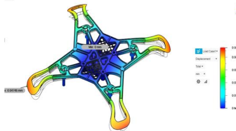
Figure 6 : ABS Plastic - Total Deformation. Figure 7 : Aluminium AlSi10Mg-Total Deformation
