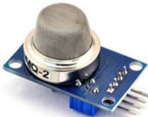
Fig : Gas Sensor
