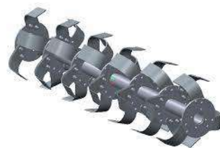
Fig. 1: Three Blade Rotavator Configuration
