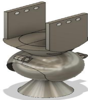
b) Ball and socket joint used as the hip joint.
