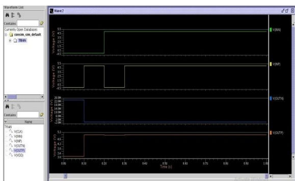
Figure 7(c): Waveforms of Conventional Double-Tail comparator
