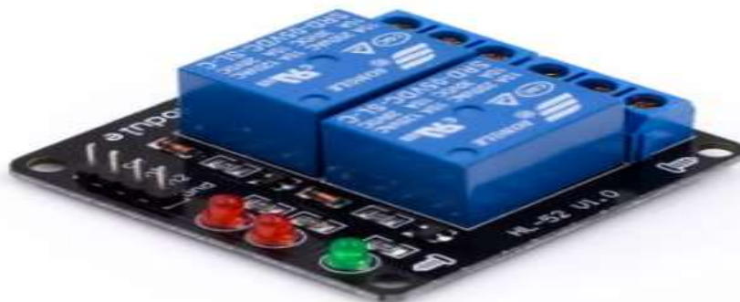
Fig 10. 5V 2 CHANNEL RELAY MODULE
