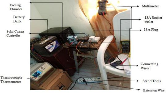
Figure 9: Experimental Setup for Solar Powered Thermoelectric Refrigerator (SPTER)
