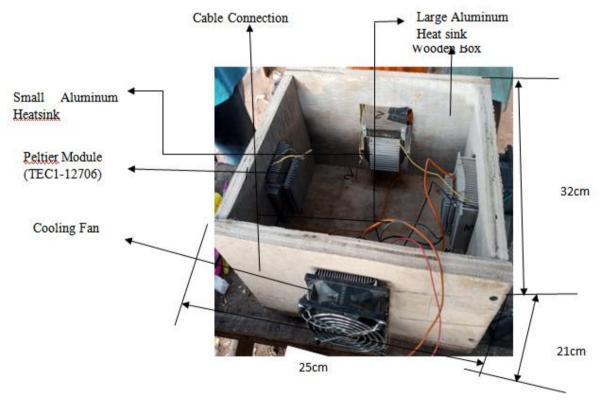
Figure 6:. Constructed wooden cooling chamber and heat sinks
