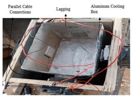
Figure 7: Constructed aluminum box with insulation
