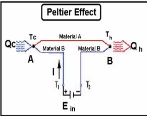
Figure1: Experimental representation of Peltier effect [3]
