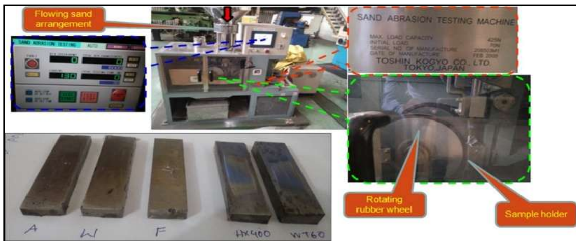
Fig 1- Dry sand- rubber wheel abrasion test machine, ToshinKogaya
