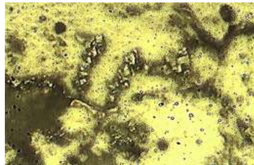
Fig. 12 Micro structural Image of SiC 6 % and ZrO 2 -2% 100x
