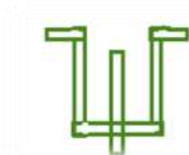
Figure 2.2: Psi ( \Psi ) Shaped Slot
