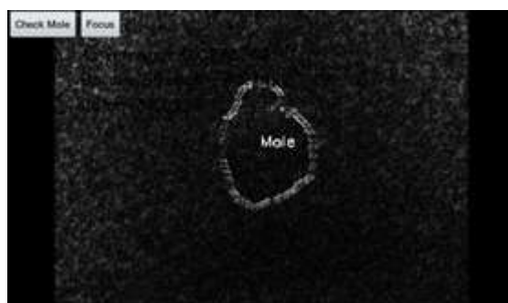
Figure 8 - Gradient magnitude map with narrow Gaussian blur. Note the dark bars within edge boundaries.
