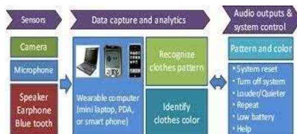
Figure2: Overview and architecture design of the camera-based clothing pattern recognition system for blind and visually impaired persons.
