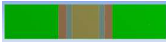
Fig 3.2 patches applied on cracks
