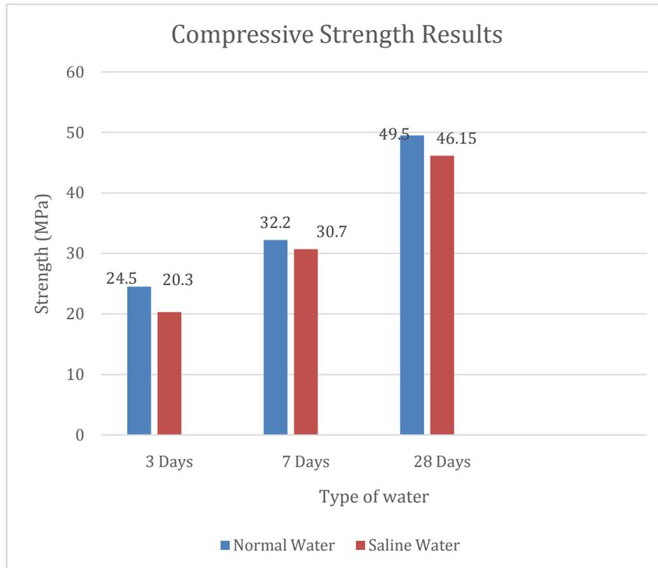
Fig:4 Compressive Strength Test
