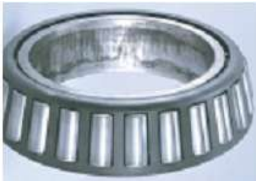
c. Wear due to friction with the ring hole in tapered roller bearings
