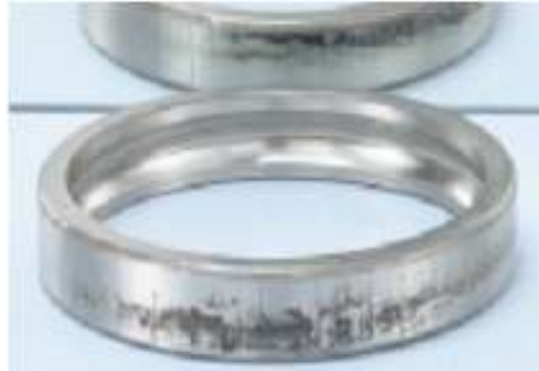
d. Wear by friction with the outer ring of the roller bearings
