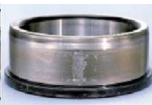
b. Pitting on the inner rings in cylindrical ball bearings
