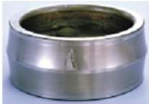
e. Pitting on the inner rings in two-row self-arranged ball bearings
