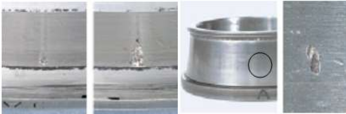
c. Pitting on the outer ring 2-row cylindrical roller bearings d. Pitting on the ring in a taper roller bearings
