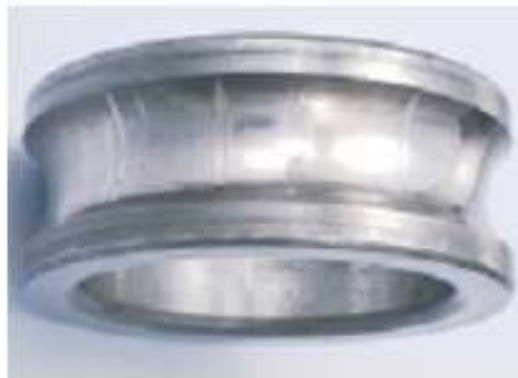
e. Wear by friction with the inner ring of the roller bearings
