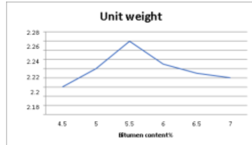
Figure 15: Unit weight for the normal mixture
