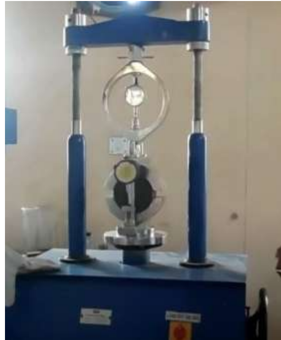
Figure 8: DBM sample testing equipment.
