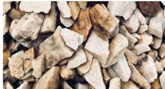
Figure 4: Crushed quartzite aggregate
