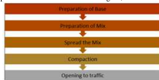
Figure 2: DBM road construction steps.
