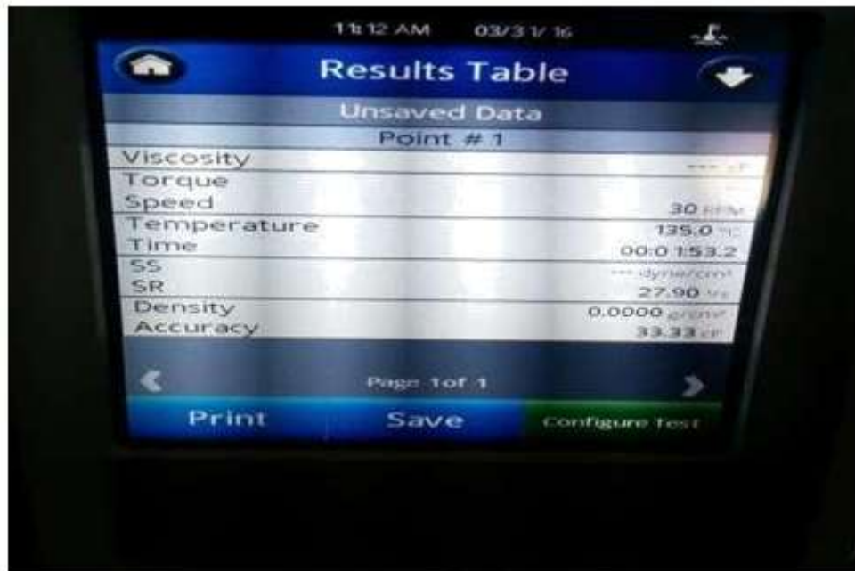
Figure 4 – Digital test result representation of viscosity.
